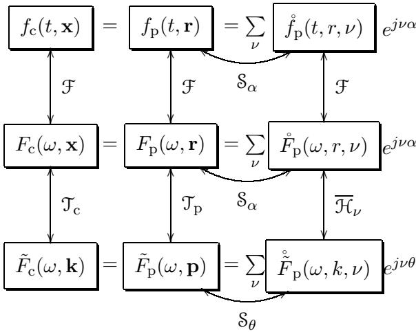
Figure 4: Representations of MD signals in the time and space domain and in the corresponding frequency domains in different coordinate systems
