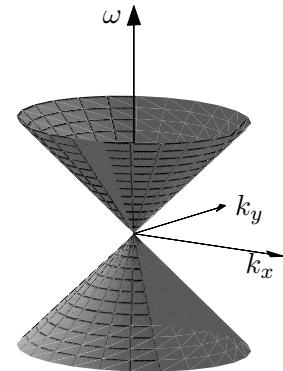
Figure 6: Support of the Dirac impulse  $\delta_c(\mathbf{k} - \mathbf{k}_0)$  in the  $(\omega, k_x, k_y)$ -domain
