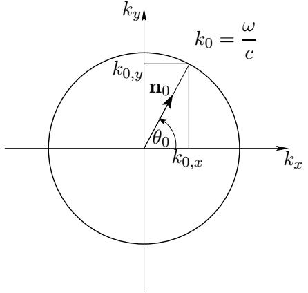
Figure 5: Possible locations of the Dirac impulse  $\delta_c(\mathbf{k} - \mathbf{k}_0)$  in the  $k_x$ - $k_y$ -plane
