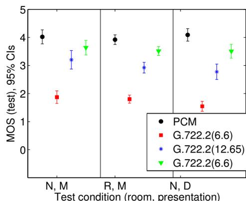
**Fig. 8:** Comparison of mean ratings for PCM, and the G.722 at 6.6, 12.65 and 23.05 kbit/s; left part: no room, monotonic; middle part: R1/R2 at 15 cm, monotonic; right part: no room, diotic.
