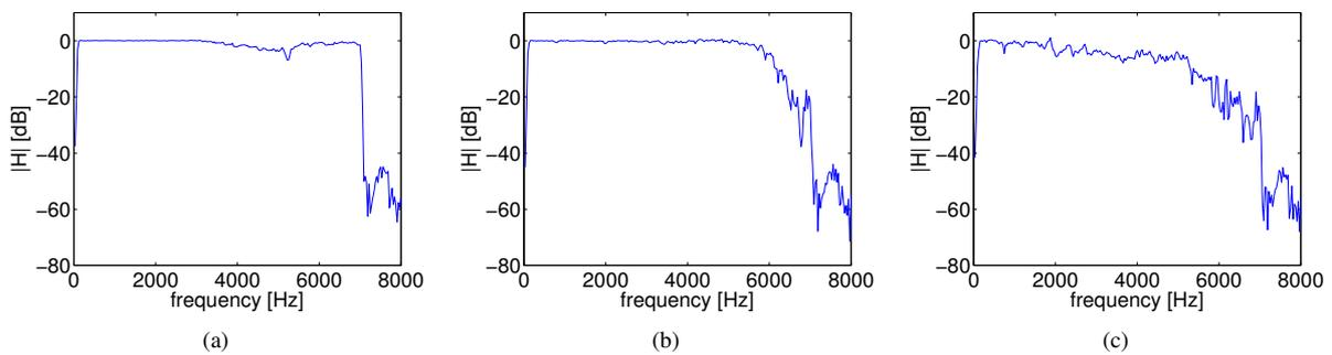
**Fig. 5:** Estimated amplitude spectra for the G.722 (64 kbit/s) (a), G.722.2 (23.05 kbit/s) (b), and G.722.2 (6.6 kbit/s) (c).
