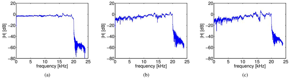
**Fig. 4:** Amplitude spectra for the Room R2 measurements, microphone at MRP (a), 15 cm (b), and 30 cm (c).
