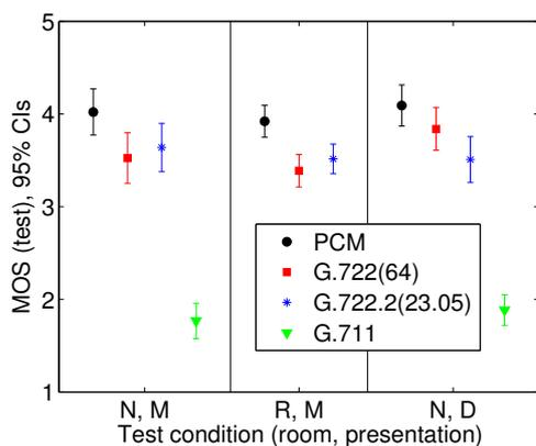
**Fig. 6:** Comparison of mean ratings for linear PCM, G.722 (64 kbit/s), G.722.2 (23.05 kbit/s) and G.711, when paired with the cases ‘no room, monotic listening (N, M; left)’, ‘room R1 or R2 at 15 cm distance, monotic (middle; R, M)’, and ‘no room, diotic (right part; N, D)’. Note that we did not test the G.711 together with a room.
