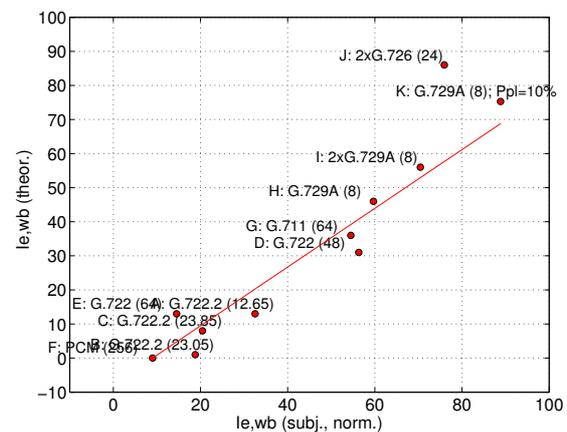
**Fig. 1:** Transformation to adjust the test results for conditions of known impairment to the values recommended in [13, 8]; the corresponding fitting-function is then applied to all test results to yield normalized values, following a method adopted from [21].
