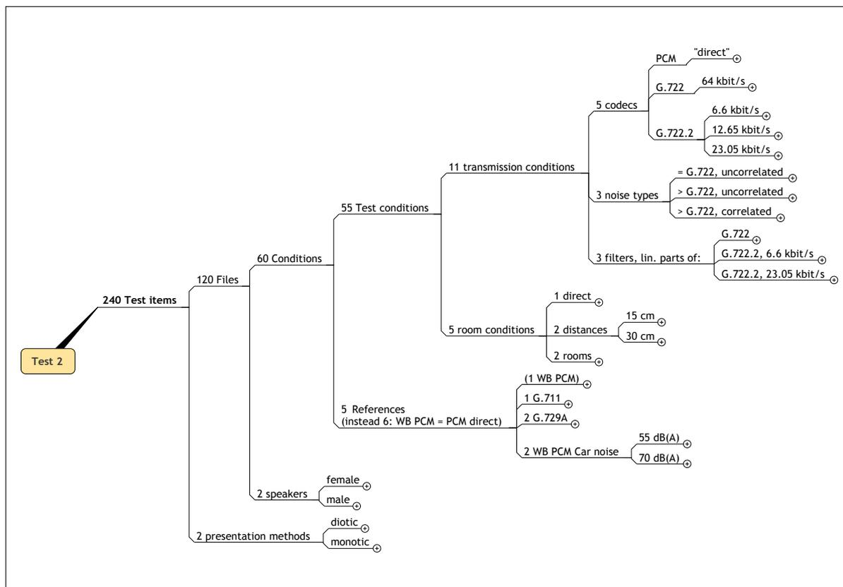
**Fig. 3:** Overview of Test 2 test conditions, see text for details.
