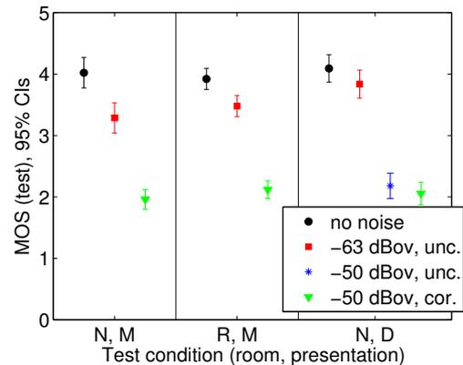
**Fig. 7:** Comparison of mean ratings for linear PCM without (no noise) and with additional codec-emulating noise (see Section 4.1) at different levels, and correlated as well as uncorrelated between the left and right channels. As in Figure 6, the left part represents the case of no room and monotic presentation, the middle part that of room at 15 cm and monotic presentation, and the right part that for diotic presentation without room.
