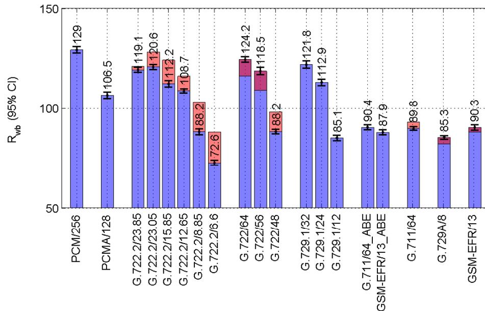
**Fig. 2:** Transformed and normalized results for error-free codecs. The blue boxes and respective errorbars show the test-results. The stacked pink and purple boxes indicate the deviation of the test results from the expected quality according to [8] and [12] (pink/errorbars below top of box: Test results lower than expected; purple/errorbars on top of box: test results higher than expected). Note: ABE indicates two NB conditions with artificial bandwidth extension.
