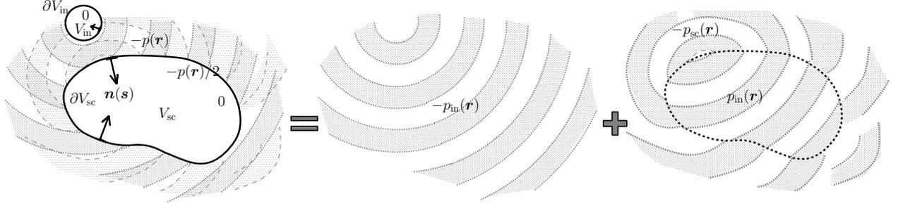
**Fig. 2:** Kirchhoff-Helmholtz integral applied to define sound-field-synthesis-equivalent sound-soft scattering on  $\partial V_{sc}$ . Here, interaction due to thinkable boundary conditions of the virtual source  $\partial V_{in}$  is neglected. The represented field must equal the original  $-p_{in}(\mathbf{r})$  plus scattered one  $-p_{sc}(\mathbf{r})$  outside  $V_{sc}$  and the perfect re-synthesis  $p_{in}(\mathbf{r})$  inside  $V_{sc}$ .
