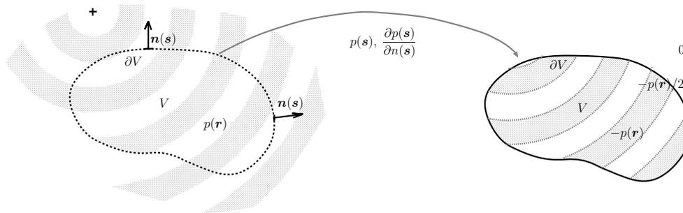
**Fig. 1:** When taking the values  $p(\mathbf{s})$  and  $\frac{\partial p(\mathbf{s})}{\partial n(\mathbf{s})}$  on a boundary  $\partial V$  around a homogeneous field, the Kirchhoff-Helmholtz integral represents  $-p(\mathbf{r})$  inside  $V$ ,  $p(\mathbf{r})/2$  on  $\partial V$ , and 0 outside.
