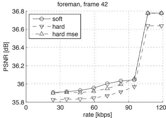
Figure 9. Last bit plane soft decoding, PSNR vs. rate for the LSB, foreman, QCIF, 30 fps,  $M = 2$
