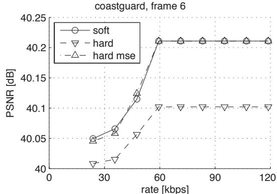
Figure 8. Last bit plane soft decoding, PSNR vs. rate for the LSB, `coastguard`, QCIF, 30 fps,  $M = 2$
