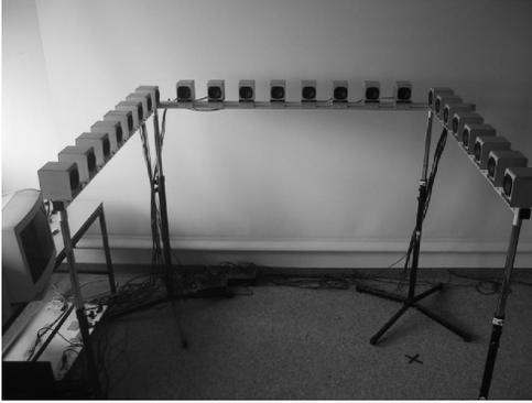
Figure 3: Typical setup of loudspeakers for WFS
