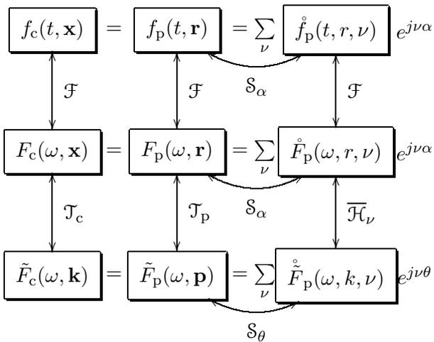
Figure 4: Representations of MD signals in the time and space domain and in the corresponding frequency domains in different coordinate systems
