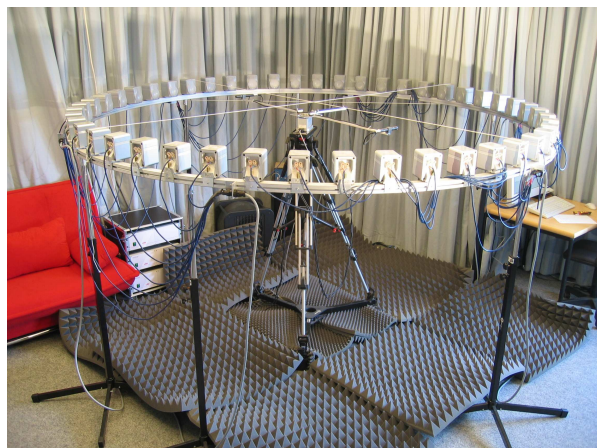
Fig. 3: Setup used for the measurement of the listening room transfer matrix. The gray curtains were removed for the measurements discussed in Section 4.2.
