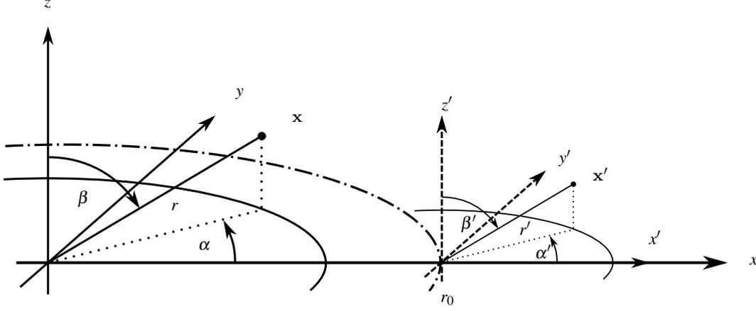
Figure 1: The coordinate systems used in this paper. Primed quantities belong to a local coordinate system at position  $\mathbf{x}'_0 = [r_0 \ 0 \ 0]^T$  (see text). The dash-dotted line indicates the secondary source distribution.
