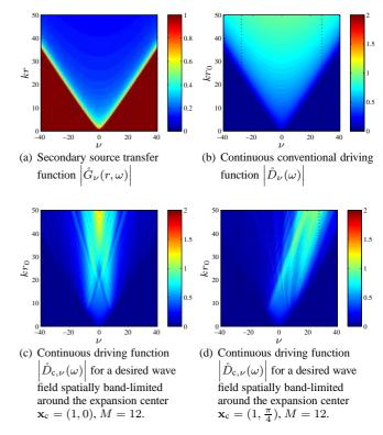
Fig. 2. Absolute values of the Fourier coefficients with respect to the expansion around the origin of the global coordinate system. The black dotted lines indicate the interval of one spectral repetition due to spatial sampling.  $kr_0=50$  corresponds to  $f\approx 2700$  Hz.
