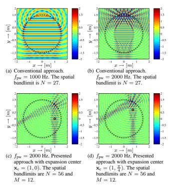
**Fig. 3.** Wave fields reproduced by a circular distribution of L=56 discrete loudspeakers and with radius  $r_0=1.5$  m reproducing a plane wave with propagation direction  $\theta_{\rm pw}=\frac{3\pi}{2}$ . The marks indicate the positions of the secondary sources.
