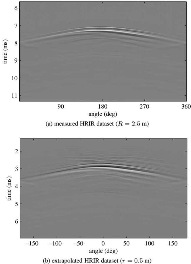
**Fig. 3:** Measured and range extrapolated HRIR dataset for the left ear ( $\alpha = 180^\circ$ ).
