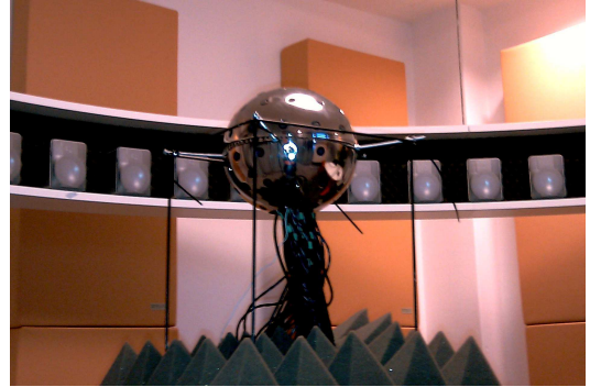
Figure 3: 56-channel loudspeaker array and 64-channel microphone array for full-duplex communication interface.
