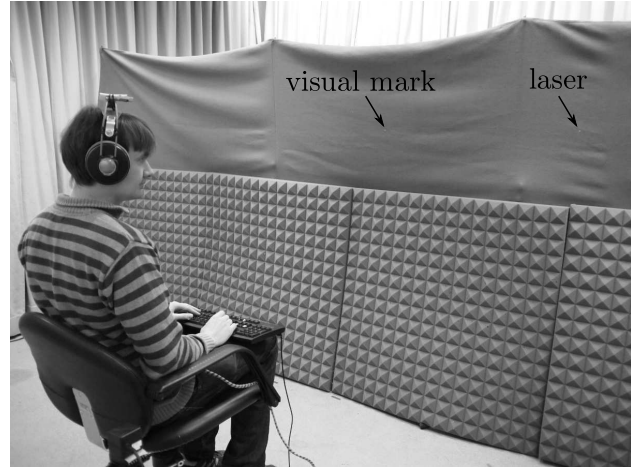
Figure 2: Sketch of the apparatus in the listening room (left) and a subject during the experiment (right). Only the blacked marked loudspeakers were used in the experiment. Note, that the room was dark during the experiment.
