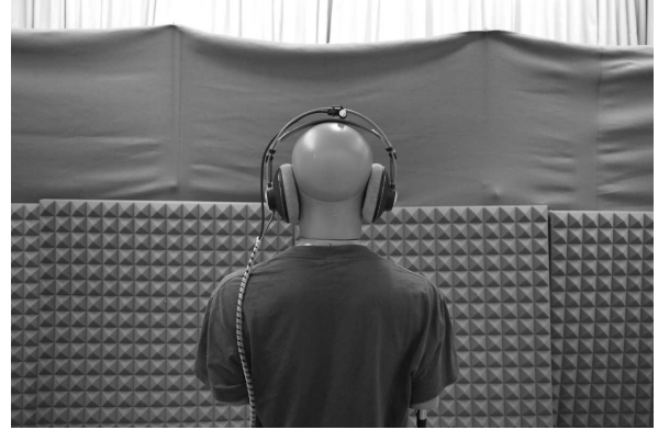
Figure 1: Measurements with the artificial head in the anechoic chamber (left) and in the listening room, which housed the experiment (right). Note, that the dummy head was wearing the same headphones as the subjects and was also suited at the same position.
