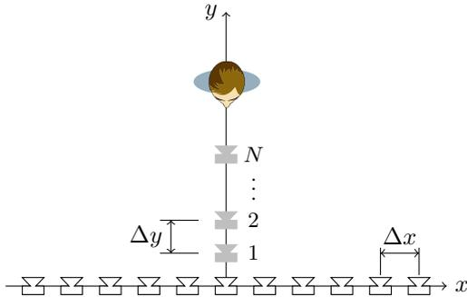
**Figure 1:** Geometry of the (virtual) endfire array.
