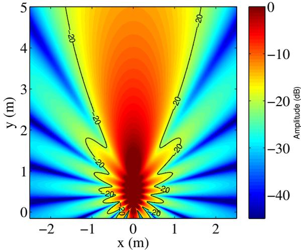
**Figure 2:** Level of monofrequent ( $f = 1000$  Hz) sound field synthesized by a superdirective endfire beamformer using point sources ( $\Delta y = 10$  cm,  $N = 8$ ,  $\beta = 10^{-6}$ ).
