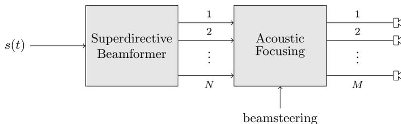
**Figure 3:** Block diagram of the two-stage approach to the generation of sound beams by a virtual endfire loudspeaker array.
