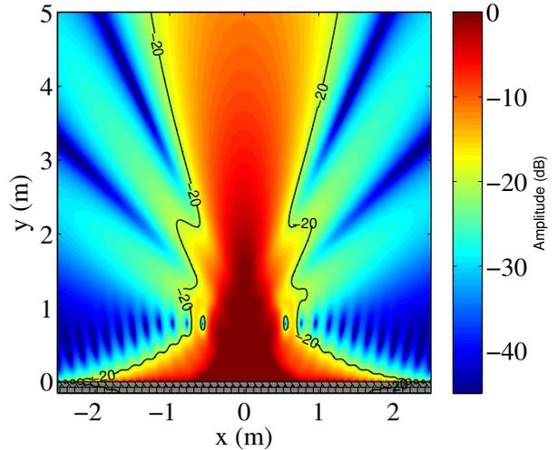
**Figure 4:** Level of monofrequent ( $f = 1000$  Hz) sound field synthesized by a virtual superdirective endfire beamformer using focused sources ( $\Delta y = 2.5$  cm,  $N = 32$ ,  $\Delta x = 10$  cm  $\beta = 10^{-6}$ ).
