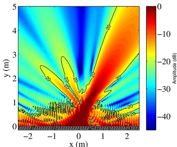
**Figure 5:** Level of monofrequent ( $f = 2000$  Hz) sound field synthesized by a virtual superdirective endfire beamformer using focused sources ( $\Delta y = 2.5$  cm,  $N = 32$ ,  $\Delta x = 10$  cm,  $\beta = 10^{-6}$ ).
