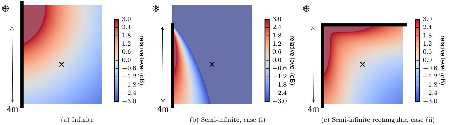
**Figure 1: 2D synthesis of a line source by secondary line sources using WFS. The edge is located at  $(0,0)$  m. The source is located at a distance of  $R = 4$  m and an angle of  $\alpha = 135^\circ$  from the reference position indicated by  $\times$ . A monochromatic source with  $f = 500$  Hz is simulated. The level is normalized to the reference position for the infinitely long secondary source distribution.**
