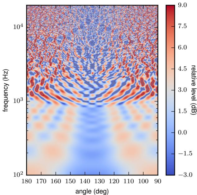
**Figure 5: Relative level at the reference position for synthesis of a point source by 2.5D WFS. The source is located at a distance of  $R = 4$  m and an angle  $\alpha$  from the reference position. The level is normalized to  $\alpha = 135^\circ$ .**
