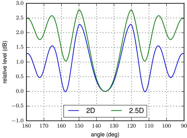
**Figure 3: 2D/2.5D synthesis by secondary line/point sources using a sampled semi-infinite rectangular secondary source distribution. Relative level at reference position for synthesis of a line/point source. A monofrequent source with  $f = 500$  Hz is simulated. The source is located at a distance of  $R = 4$  m and angle  $\alpha$  from the reference position. The level is normalized for  $\alpha = 135^\circ$ .**
