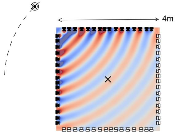
**Figure 4: 2.5D synthesis of a monochromatic point source by WFS. The source is located at a distance of  $R = 4$  m and angle  $\alpha = 135^\circ$  from the reference position indicated by  $\times$ . A monochromatic source with  $f = 500$  Hz is simulated. The level is normalized to the reference position for  $\alpha = 135^\circ$ .**
