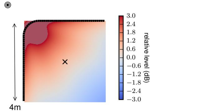
(a) relative level of synthesized sound field for  $N_r = 10$ ,  $\alpha = 135^\circ$
