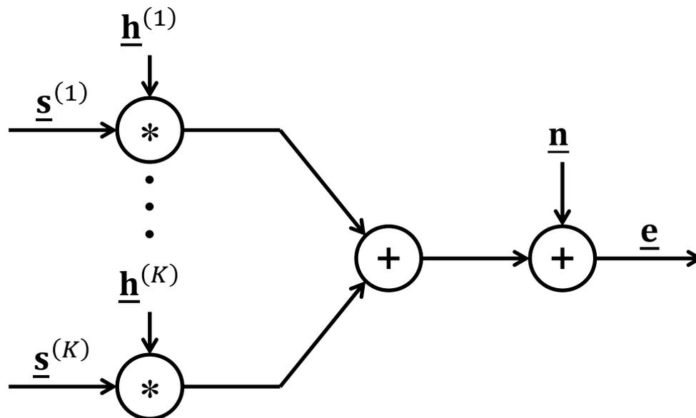
$$\underline{\mathbf{e}} = \sum_{k=1}^K \underline{\mathbf{G}}^{(k)} \cdot \underline{\mathbf{h}}^{(k)} + \underline{\mathbf{n}} = \underbrace{\left( \underline{\mathbf{G}}^{(1)} \quad \dots \quad \underline{\mathbf{G}}^{(K)} \right)}_{\underline{\mathbf{G}}} \cdot \underbrace{\begin{pmatrix} \underline{\mathbf{h}}^{(1)} \\ \vdots \\ \underline{\mathbf{h}}^{(K)} \end{pmatrix}}_{\underline{\mathbf{h}}} + \underline{\mathbf{n}}$$
