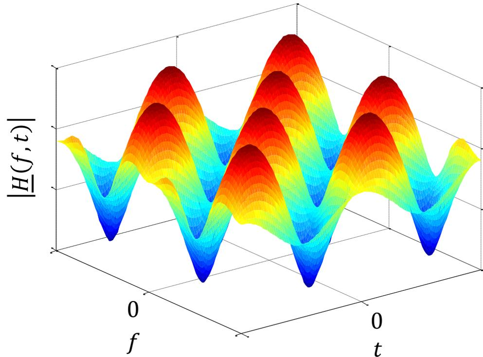
$$\begin{aligned} \underline{H}(f, t) = & \underline{h}_0 e^{-j2\pi f \tau_0} e^{j2\pi f D_{,0} t} \\ & + \underline{h}_1 e^{-j2\pi f \tau_1} \\ & + \underline{h}_2 e^{-j2\pi f \tau_2} e^{j2\pi f D_{,2} t} \end{aligned}$$
