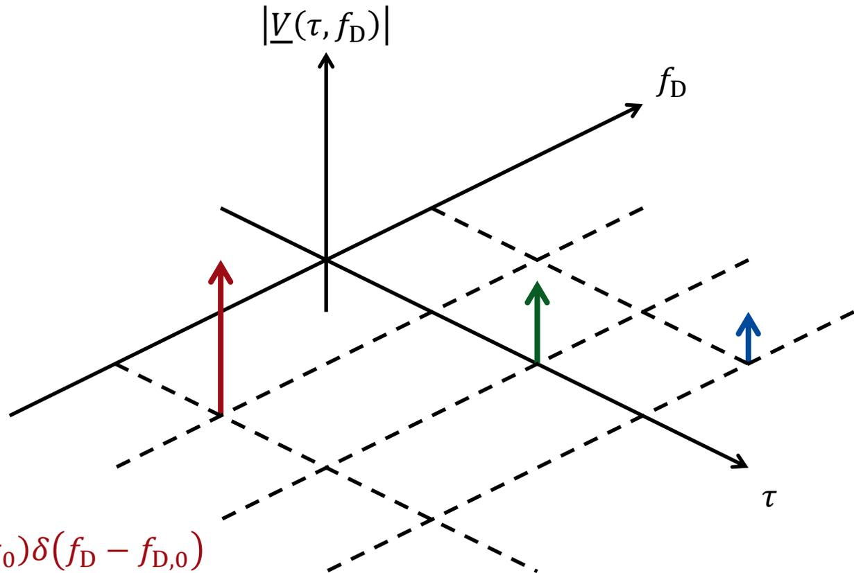
$$\begin{aligned} \underline{V}(\tau, f_D) = & \underline{h}_0 \delta(\tau - \tau_0) \delta(f_D - f_{D,0}) \\ & + \underline{h}_1 \delta(\tau - \tau_1) \delta(f_D) \\ & + \underline{h}_2 \delta(\tau - \tau_2) \delta(f_D - f_{D,2}) \end{aligned}$$
