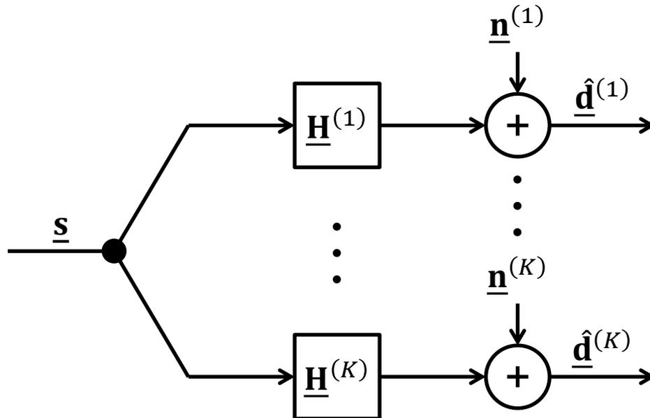
$$\underbrace{\begin{pmatrix} \hat{\underline{d}}^{(1)} \\ \vdots \\ \hat{\underline{d}}^{(K)} \end{pmatrix}}_{\underline{\hat{d}}} = \underbrace{\begin{pmatrix} \underline{H}^{(1)} \\ \vdots \\ \underline{H}^{(K)} \end{pmatrix}}_{\underline{H}} \cdot \underline{s} + \underbrace{\begin{pmatrix} \underline{n}^{(1)} \\ \vdots \\ \underline{n}^{(K)} \end{pmatrix}}_{\underline{n}}$$
