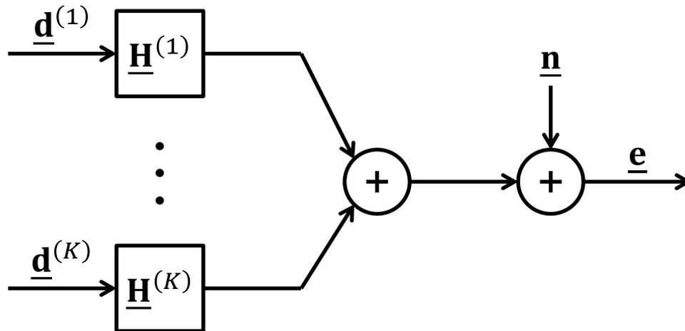
$$\begin{aligned} \underline{e} &= \sum_{k=1}^K \underline{H}^{(k)} \cdot \underline{d}^{(k)} + \underline{n} \\ &= \underbrace{\left( \underline{H}^{(1)} \quad \dots \quad \underline{H}^{(K)} \right)}_{\underline{H}} \cdot \underbrace{\begin{pmatrix} \underline{d}^{(1)} \\ \vdots \\ \underline{d}^{(K)} \end{pmatrix}}_{\underline{d}} + \underline{n} \end{aligned}$$
