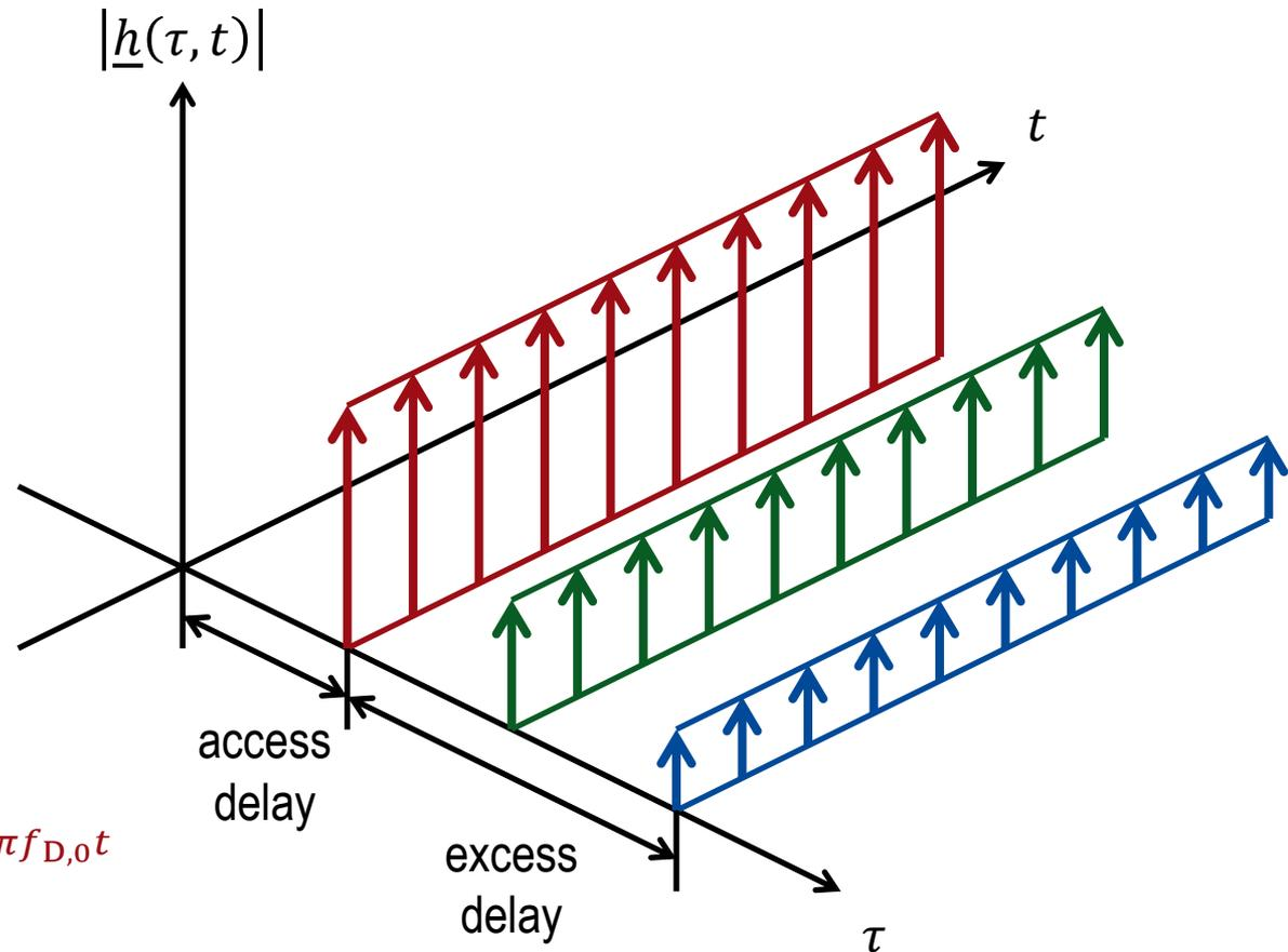
$$\begin{aligned} \underline{h}(\tau, t) = & \underline{h}_0 \delta(\tau - \tau_0) e^{j2\pi f_{D,0}t} \\ & + \underline{h}_1 \delta(\tau - \tau_1) \\ & + \underline{h}_2 \delta(\tau - \tau_2) e^{j2\pi f_{D,2}t} \end{aligned}$$
