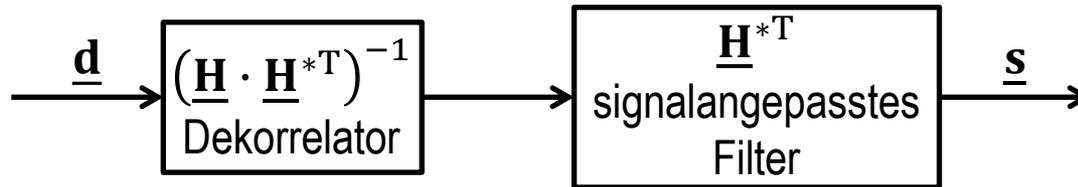
$$\hat{\underline{d}} = \underline{\mathbf{H}} \cdot \underline{\mathbf{M}}_{\text{ZF}} \cdot \underline{\mathbf{d}} + \underline{\mathbf{n}} = \begin{bmatrix} 1 & & & & \\ & 1 & & & \\ & & 1 & & \\ & & & 1 & \\ & & & & 1 \end{bmatrix} \cdot \underline{\mathbf{d}} + \underline{\mathbf{n}}$$
