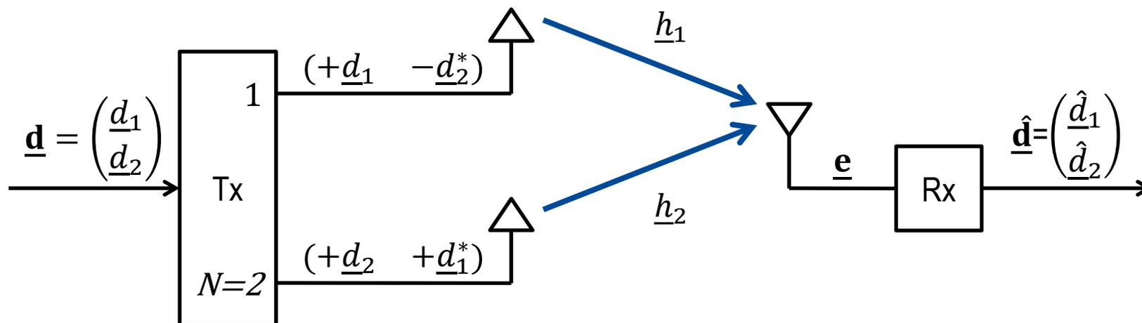
$$\underbrace{\begin{pmatrix} \underline{e}_1 \\ \underline{e}_2^* \end{pmatrix}}_{\underline{e}} = \underbrace{\begin{pmatrix} \underline{h}_1 & \underline{h}_2 \\ \underline{h}_2^* & -\underline{h}_1^* \end{pmatrix}}_{\underline{H}} \cdot \underbrace{\begin{pmatrix} \underline{d}_1 \\ \underline{d}_2 \end{pmatrix}}_{\underline{d}} + \underbrace{\begin{pmatrix} \underline{n}_1 \\ \underline{n}_2^* \end{pmatrix}}_{\underline{n}}$$
