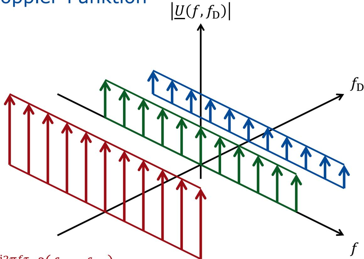
$$\begin{aligned} \underline{U}(f, f_D) = & \underline{h}_0 e^{-j2\pi f \tau_0} \delta(f_D - f_{D,0}) \\ & + \underline{h}_1 e^{-j2\pi f \tau_1} \delta(f_D) \\ & + \underline{h}_2 e^{-j2\pi f \tau_2} \delta(f_D - f_{D,2}) \end{aligned}$$
