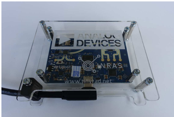
Figure 2: TinyRad radar sensor from Analog Devices. Reverse side with the electronics.
